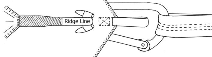
Pull carabiner tight and attach to the tree strap, then repeat at the other end. Now adjust tension to keep the ridgeline taught and level, or you may adjust for your head to be slightly higher or lower than your feet.
